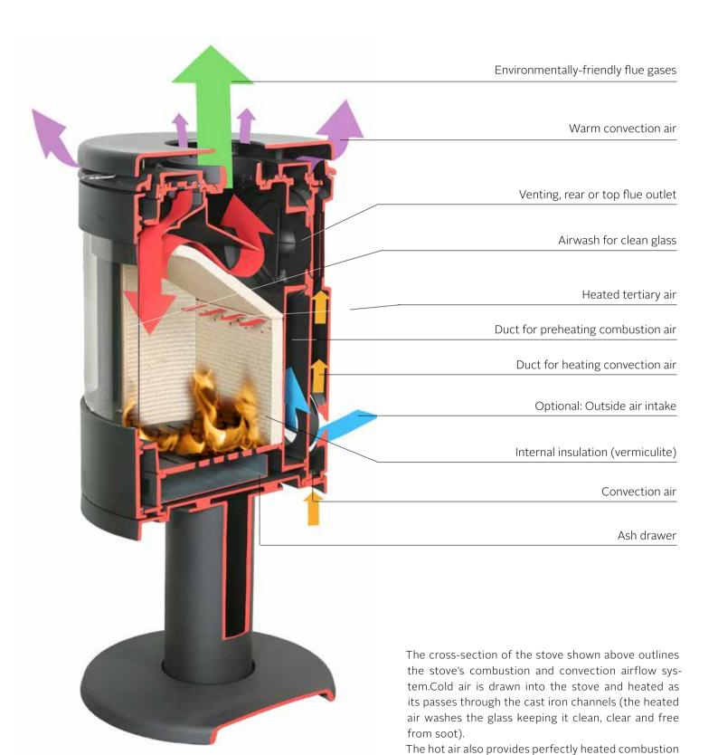
air (in addition the heated tertiary air aids secondary combustion of any smoke and gasses, increasing efficiency and reducing the environmental impact).
