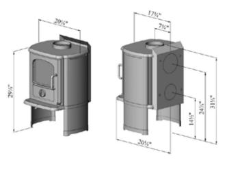
Maximum Heat . . . . 30,000 BTU/hr Max. Area Heated . . . . . 1000 ft<sup>2</sup> Firebox Dimensions 131/4" W x 121/2" D Firebox volume/capacity . . . . 0.9 ft<sup>3</sup> Outside air supply . . . . . Available Mobile home approved . . . . . Yes
